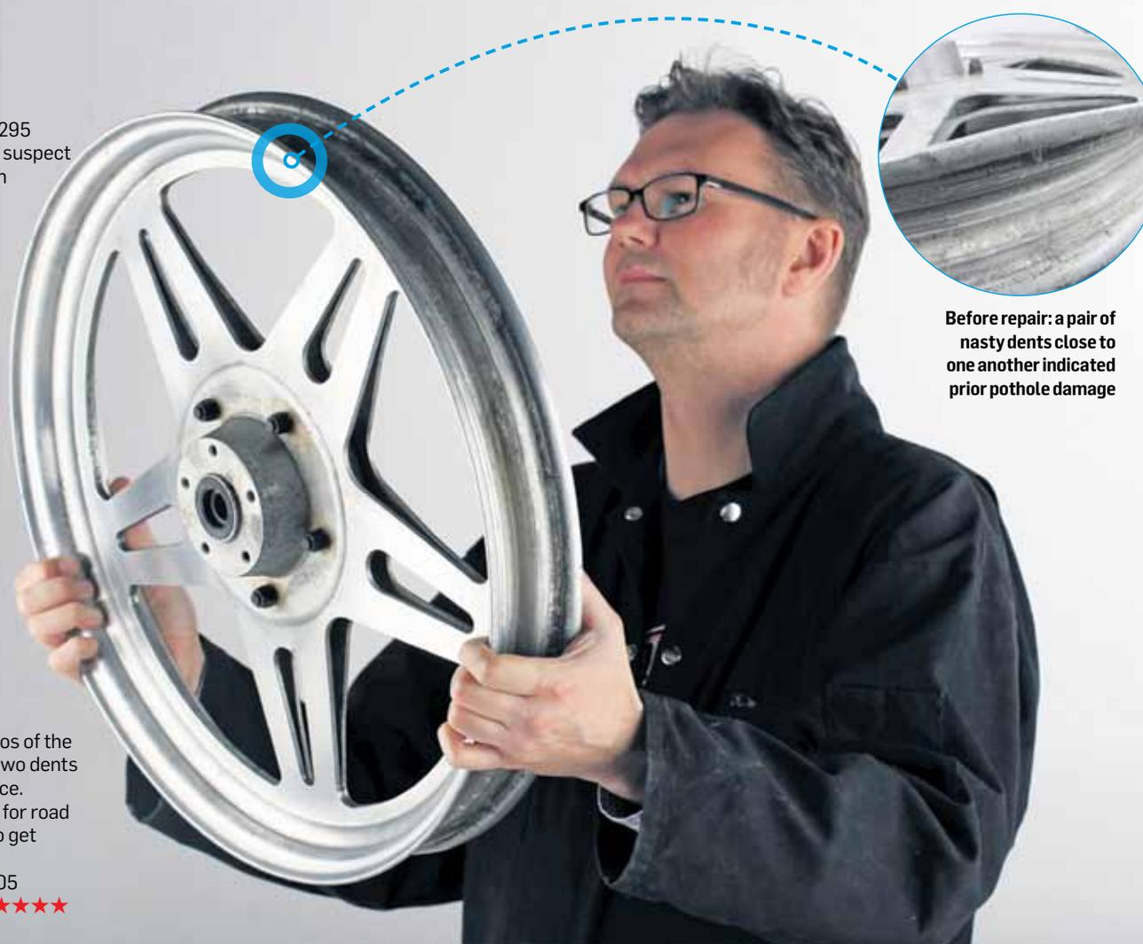
Before repair: a pair of nasty dents close to one another indicated prior pothole damage
