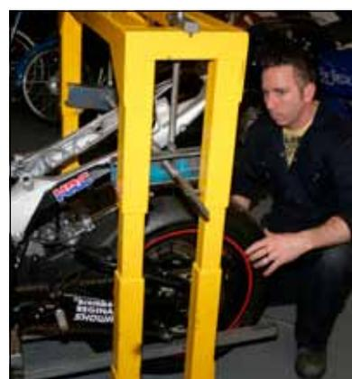
**Top:** Ray (left) and son Tommy Palmer with a recently restored 50cc Itom Mk8. **Above:** Tommy clamping a frame in one of the jigs prior to straightening. **Left:** An Inclinometer gives a preliminary indication of the extent of damage to the frame
